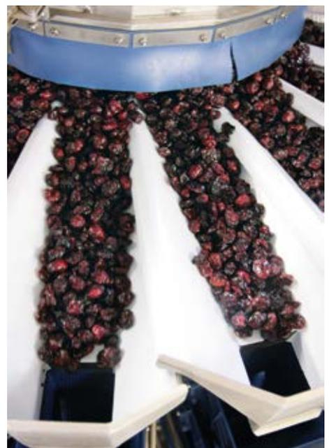
**A**s a result, two additional MP 20-1000-400-H-S5 MULTIPOND multihead weighers have recently been purchased. The purpose of the acquisition was to be able to guarantee precise ratios for nut and dried fruit mixtures.
